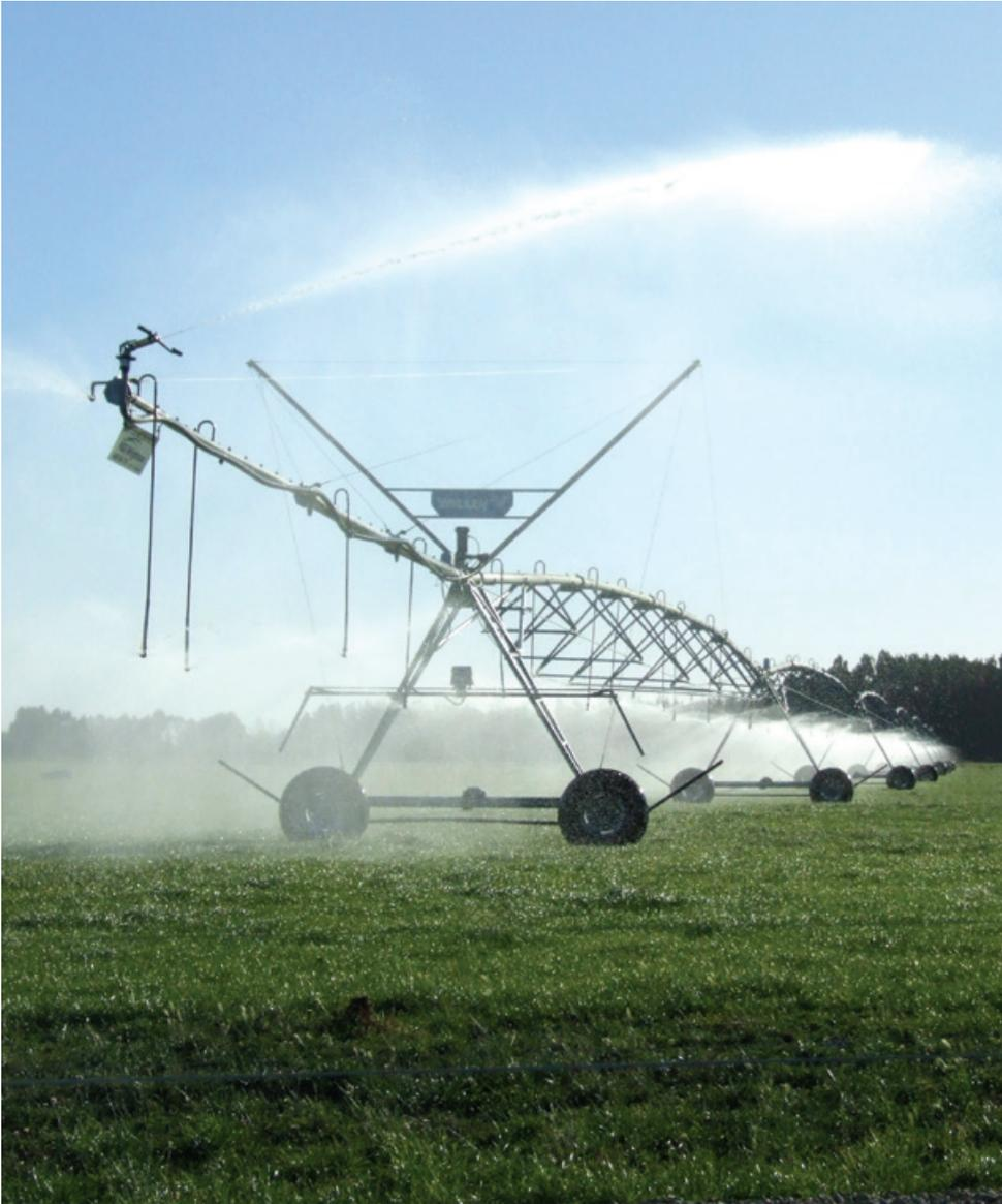
A single blocked nozzle on a centre pivot can cause several hectares of grass to die off in a short space of time. Alternatively, rotation and application rates of centre pivots if not managed accurately, can saturate your paddocks and lead to expensive water evaporating into thin air.
